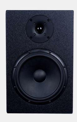
**Frequency Range** 48Hz-20kHz (-6dB) In Room Response **Power Handling** 50-150 Watts recommended amplifier power Sensitivity 90dB for 2.83 volts at 1 meter **Impedance**  $8\Omega$  (minimum  $4\Omega$ ) Configuration 2 way **Enclosure Type** Bass reflex, front vented Driver Low Frequency Driver-Single 8" paper cone driver High Frequency Driver-25mm (1") Silk Dome Tweeter **Input Terminal**
